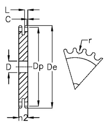
C = 4 D = 30 De = 520.8 Dp = 505.65 For chain size = 1 1/4 x 3/4 For chain type = 20 B-2 h2 = 54.6
